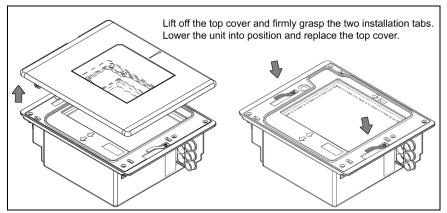
Figure 12: Installation Tabs
