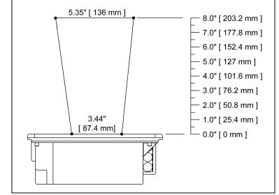
Figure 29: Scan Volume in Plane Perpendicular to Flow
