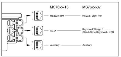
Figure 33: Scanner Interface Ports
