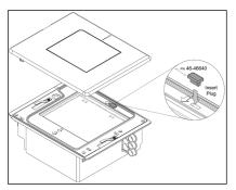
Figure 17: POS Plug Installation
