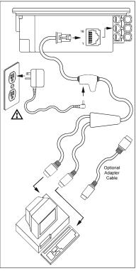
Figure 15: Keyboard Wedge Interfaces
