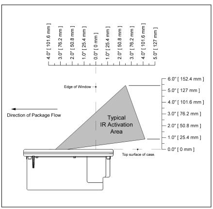
Figure 28: IR Activation Area Parallel to Package Flow
