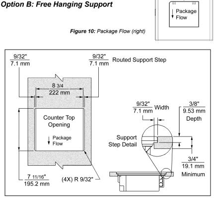
Figure 11: Specifications for Free Hanging Support
