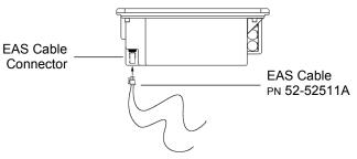
Figure 24: EAS Cable and Connector
