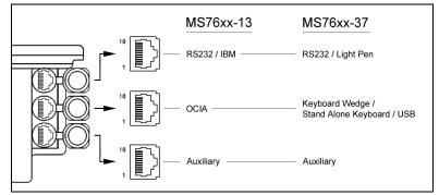
Figure 32: Scanner Interface Ports
